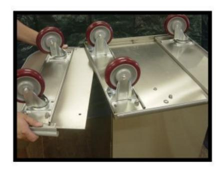
3 Insert plate into seam.
