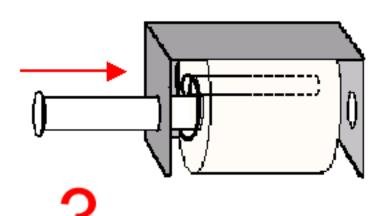
Push Tube through Frame opening and through the Loop of Tension Adapter.
