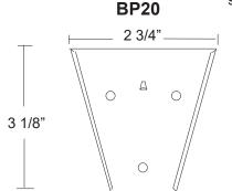
Three 3/16" mounting holes on wall bracket. See mounting instructions.
